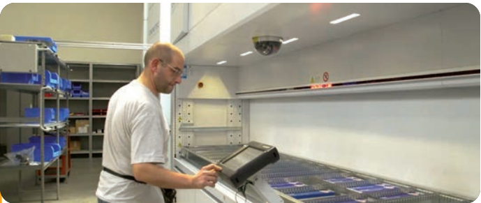
Put-to-light systems connected to WMS
