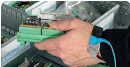
ESD Protection System
